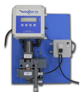
The Series RAH-210 Analyzer makes use of the Amperometric method to determine residual levels in the sample water. The measurement cell consists of large anodic and cathodic electrodes in direct contact with the sample water. The measurement is continuous, not relying on sample and hold methods, thereby allowing for better process control. A continuously driven cleaning system is employed to prevent the build up of impurities on the surface of the electrodes and reduce the need for maintenance.
